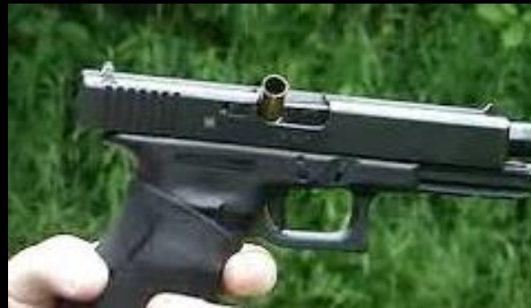
Failure to eject
