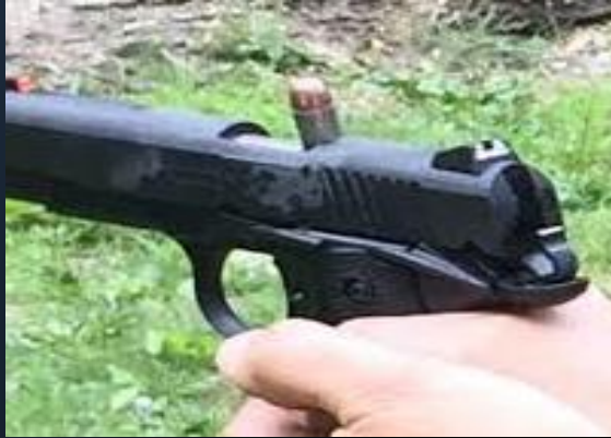
Failure to feed
